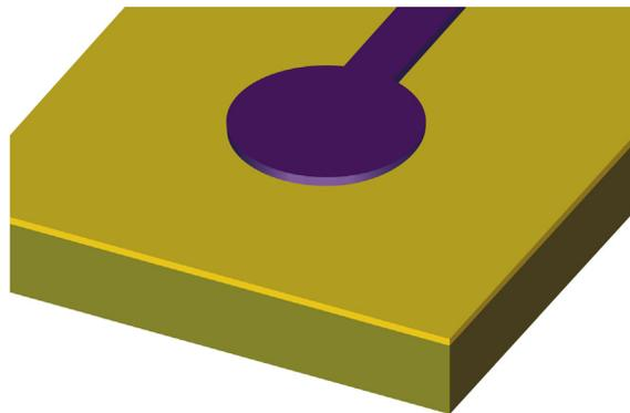
**Figure 1.9** Developed photoresist on copper.
