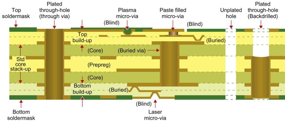
**Figure 1.5** A built-up, multitechnology, PCB stack-up. *PCB*, Printed circuit board.
