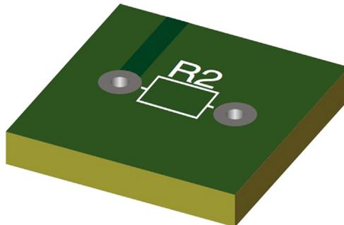
**Figure 1.16** Final layers are the soldermask [*dark green* (dark gray in print version)] and silk screen (*white*).
