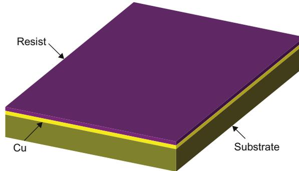
**Figure 1.6** A copper clad board coated with photoresist.
