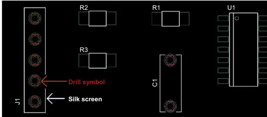
Figure 1.18 Circuit layout with drill symbols and silk screen on a PCB.
