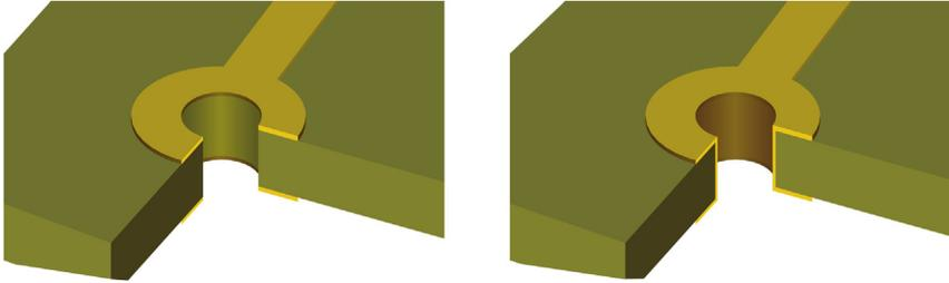
**Figure 1.13** Holes are drilled into the board and copper plated: (left) a nonplated through hole and (right) a plated through hole.
