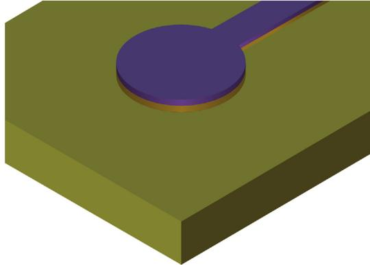
**Figure 1.10** Unwanted copper removed by etching.
