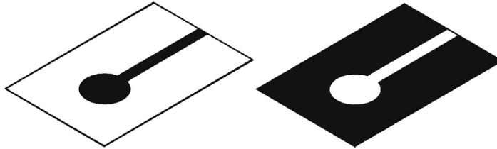
**Figure 1.7** Photolithography masks: (left) positive mask and (right) negative mask.
