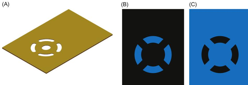
**Figure 1.21** Copper in a plane layer: (A) copper plane with thermal relief, (B) negative view as processed, and (C) displayed in WYSIWYG mode. *WYSIWYG*, What you see is what you get.
