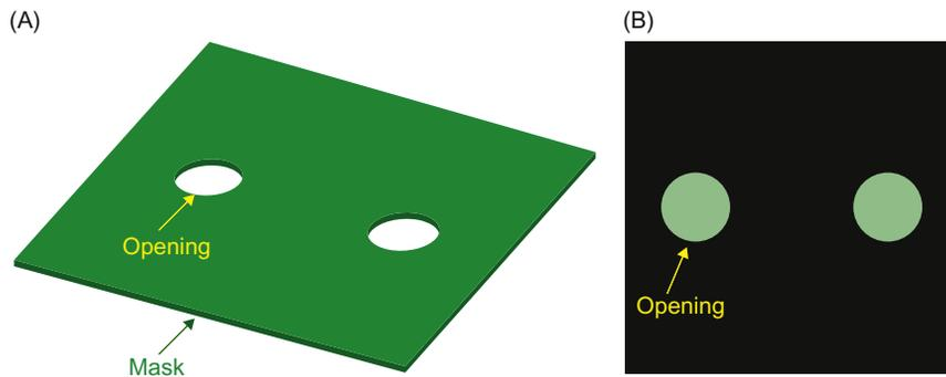
Figure 1.20 Soldermask layer and negative view: (A) soldermask and (B) negative view in PCB Editor.
