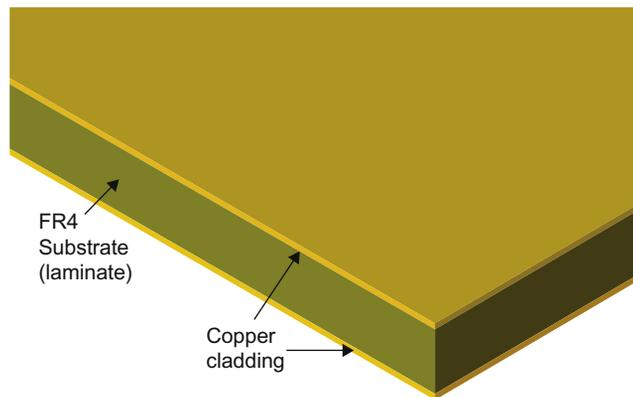
Figure 1.2 A double-sided copper clad FR4 substrate.
