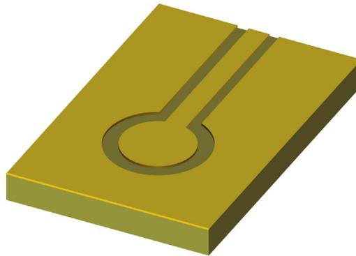
**Figure 1.12** A mechanically milled trace.
