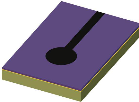
**Figure 1.8** Positive photomask on photoresist-coated board.
